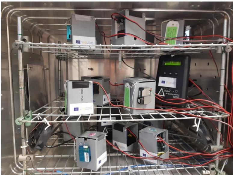
*Figure 1: Exposure box used for PM testing with the three grids visible*
