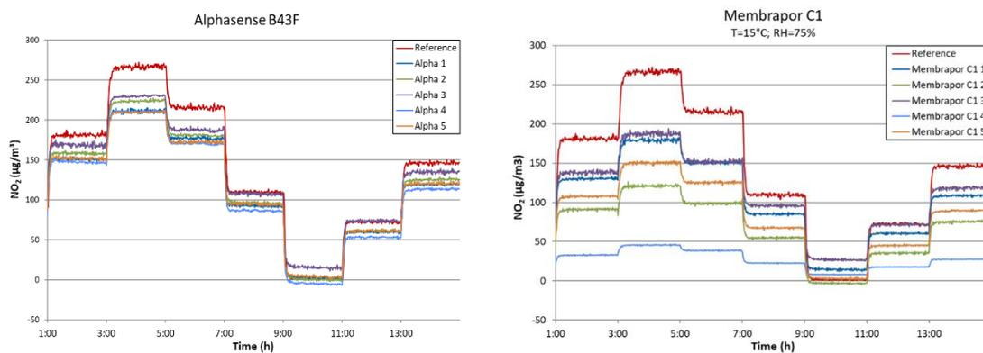
Figure 1 Examples of sensors' responses (Alphasense and Membrapor C1) compared to the reference instrument (indicated in red) during the ramping experiment; time resolution: one minute
