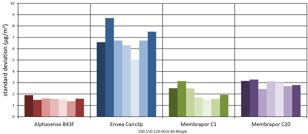
Figure 5 Standard deviation of the NO<sub>2</sub> sensors for each of the seven concentration levels of the ramping experiment; for each sensor the right bar is the average value
