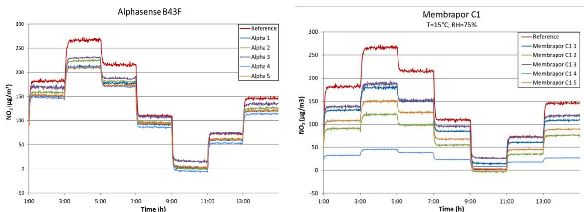
Figure 4 Examples of sensors' (Alphasense and Membrapor C1) responses in the ramping experiment after calibration; time resolution: one minute, reference indicated in red
