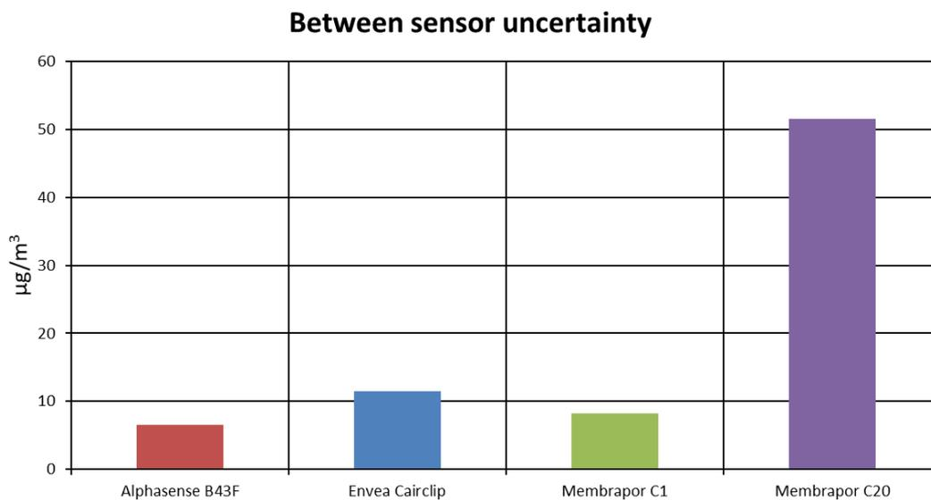
Figure 6 Between sensor uncertainty for each sensor system
