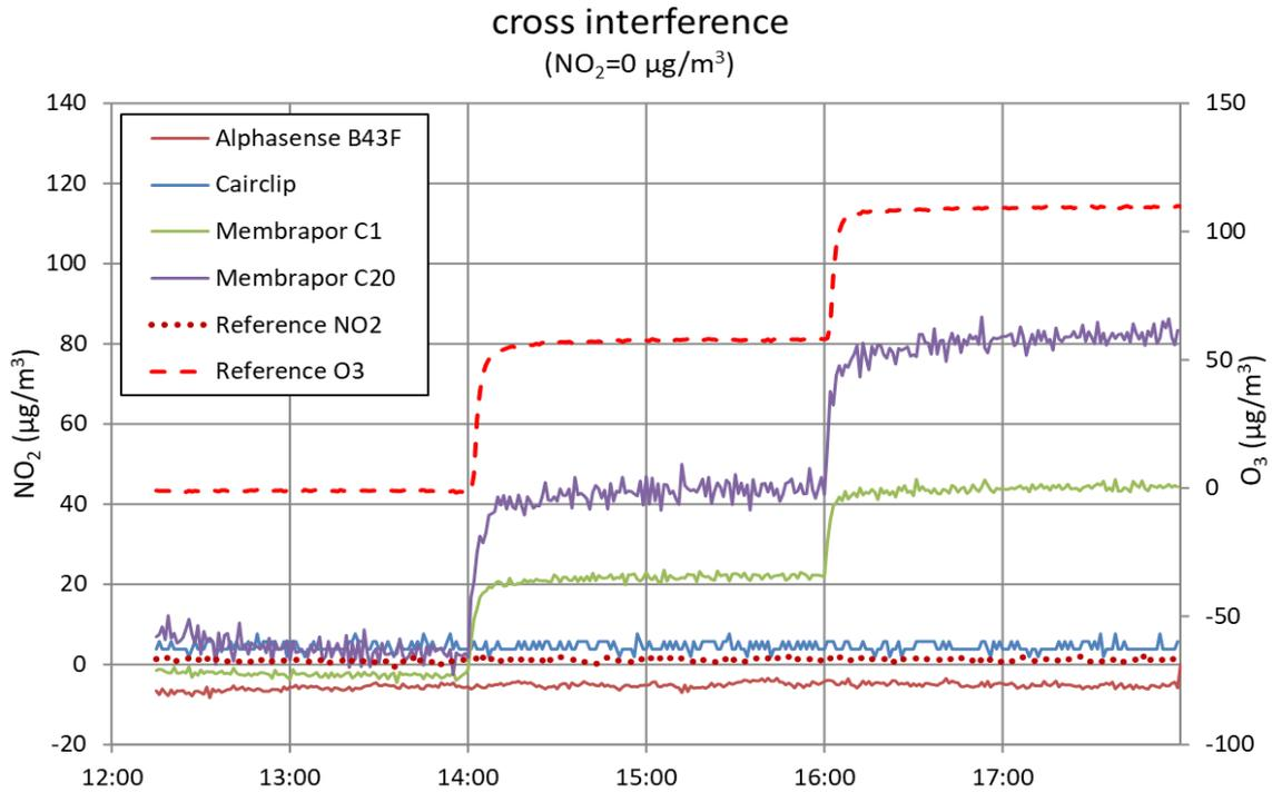
Figure 9 Response of NO<sub>2</sub> sensors at different levels of O<sub>3</sub> (with NO<sub>2</sub> = 0 µg/m<sup>3</sup>)
