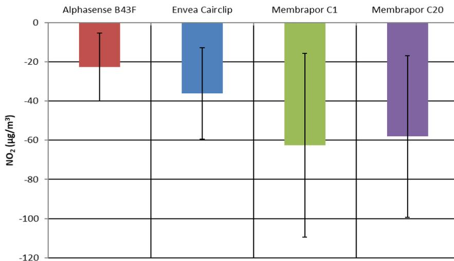
Figure 2 Average deviation (per sensor system) from the average reference concentration during the ramping experiment
