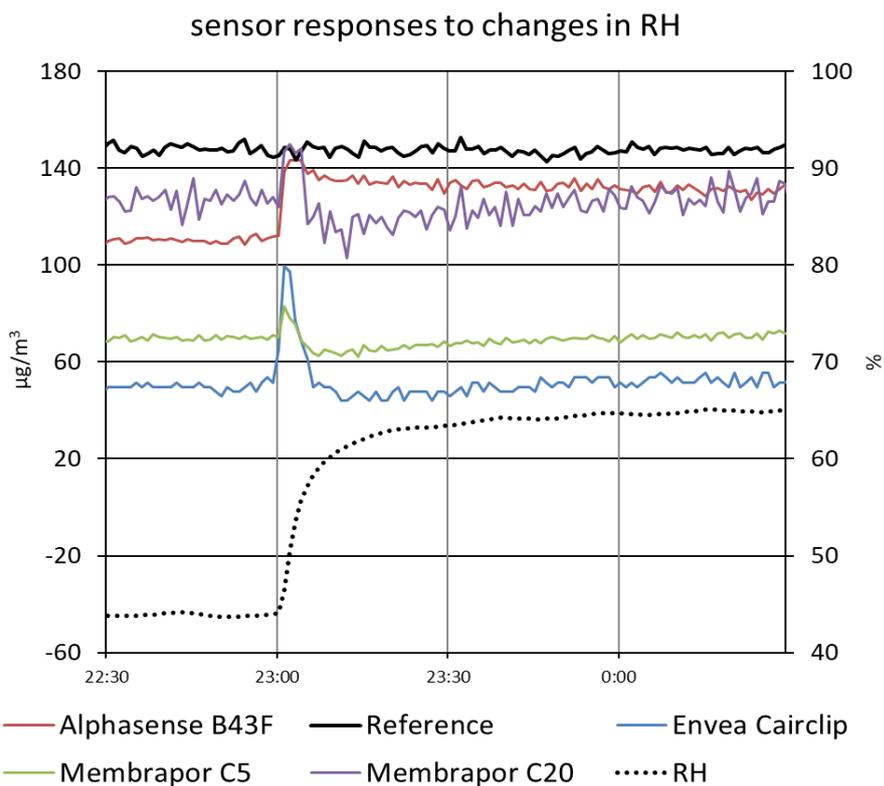
Figure 8 Responses of various NO<sub>2</sub>-sensors when increasing RH (at fixed T and NO<sub>2</sub>)
