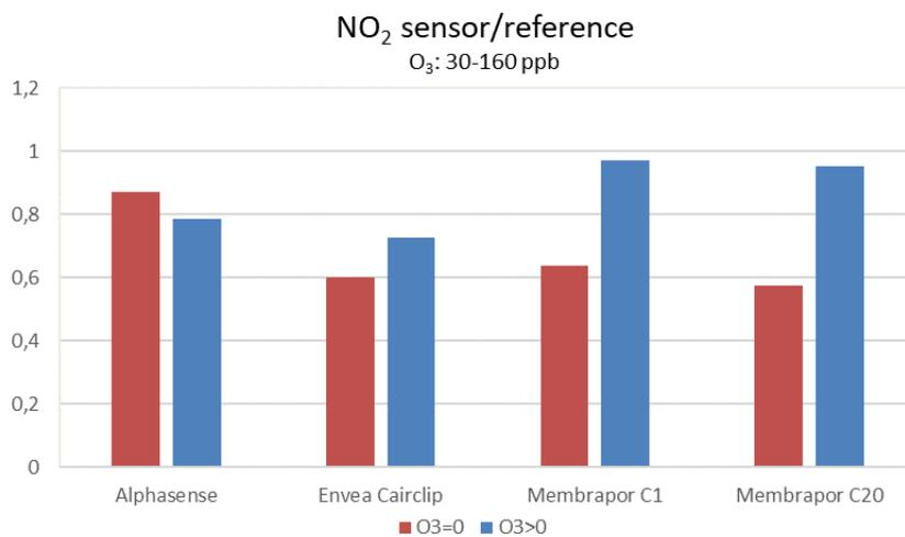
Figure 10 Ratios sensor versus reference (per sensor) with NO<sub>2</sub>>0 (and O<sub>3</sub>=0 or O<sub>3</sub>>0)
