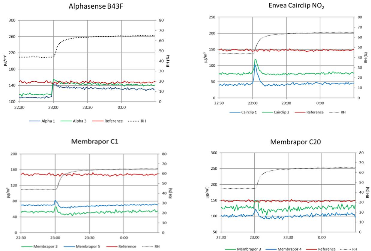
Figure 7 Responses of NO<sub>2</sub>-sensors due to a step change in RH (at fixed T and NO<sub>2</sub>)
