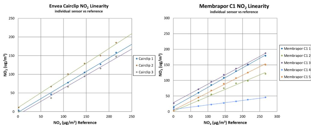
Figure 3 Examples of linearity (Envea Cairclip and Membrapor C1)
