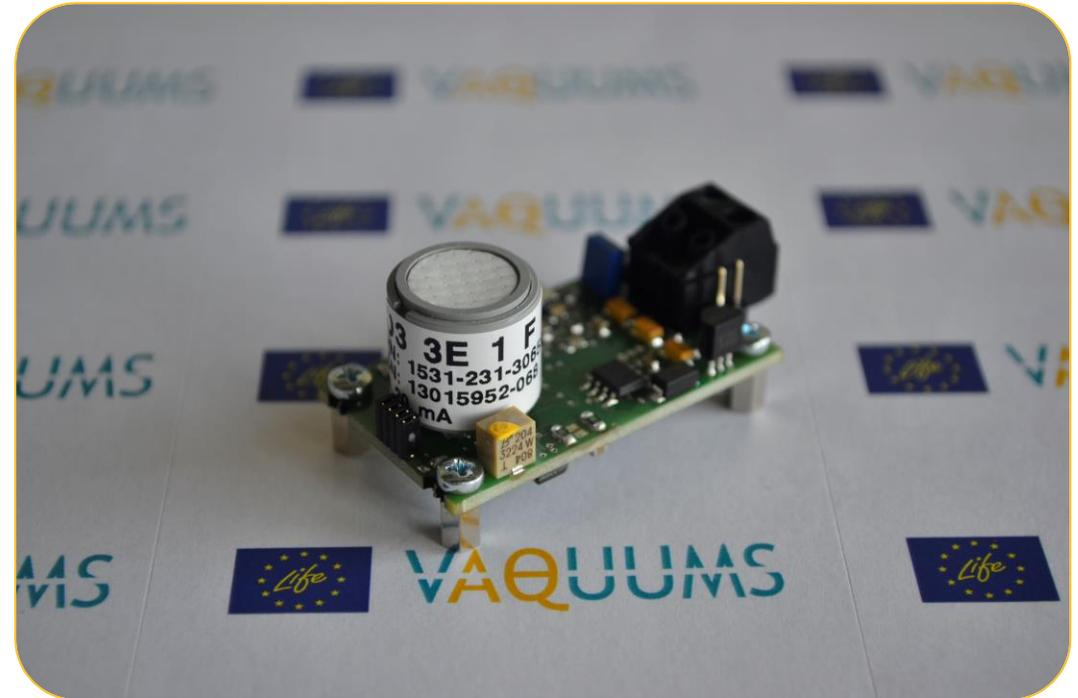
The Citytech O3 3E1F is an electrochemical ozone sensor. According to the manufacturer it can measure concentrations between 0 and 1 ppm, with a resolution of 0.03 ppm. It is mostly used for industrial applications.
